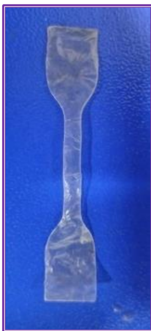
Figure 4: Showing the Dumbbell Shaped Sample
