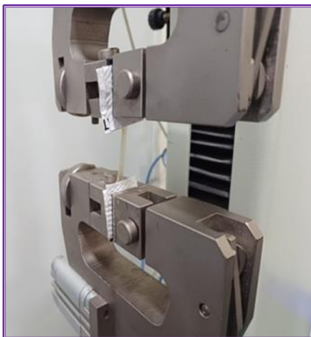
Figure 5: Showing the Dumbbell Shaped Sample Fixed Between the Two Grips of Universal Testing Machine
