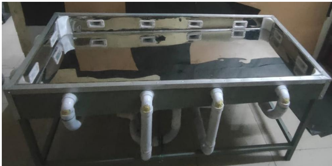
Fig.1 Cadaver Table with Local Exhaust Ventilation
